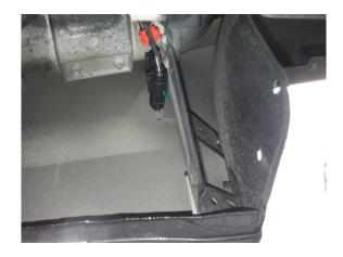
9a) Connect red to purple (purple on truck) 9b) Connect Black to Brown (brown on truck) Some New Trucks have different coloured wires. Connect Red to Yellow (Yellow On Truck) **Connect Black to White (White on Truck)**
