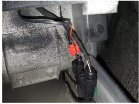
5) Feed Cables out of tailgate and strap tight using cable ties, Feed out towards the side the fuel filler cap is.
